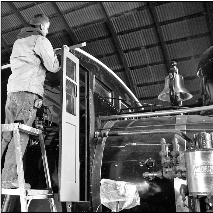
Finishing touches are put on the newly built wooden cab for C&S #9 at Uhrich Locomotive Works in Strasburg, Colorado, on 4/28/06. – Photo © Dave Schaaf.
